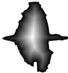
Figure 1.11: Distance map using stretched grayscale values for display. The center of the image is the background.
