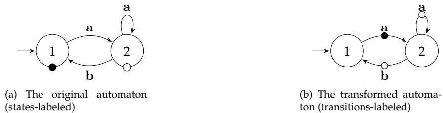
Figure 3.3: An automaton with labels on states into an automaton with labels on transitions.
